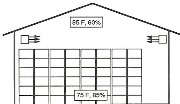
Figure 1. Curing room with top mounted heaters. Numbers in boxes are typical air temperature and relative humidity in the top and bottom portions of the room.
