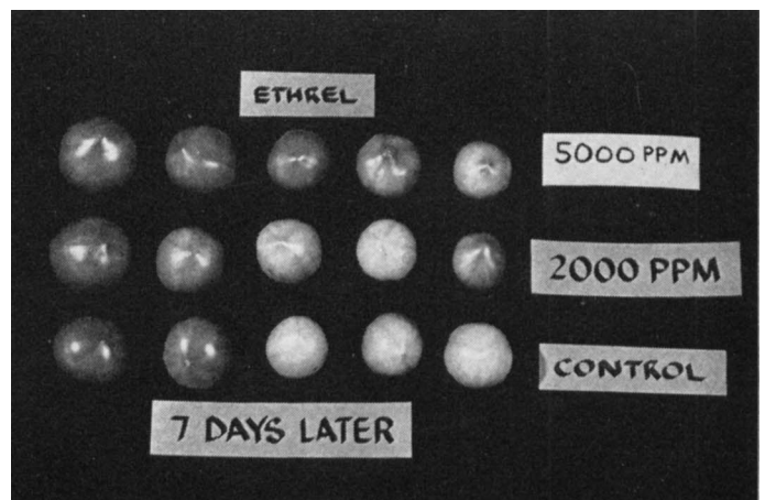
Photo 5. Ripening seven days after mature green fruits had been dipped for 30 seconds in Ethrel at concentrations of 5,000, 2,000, and control.
