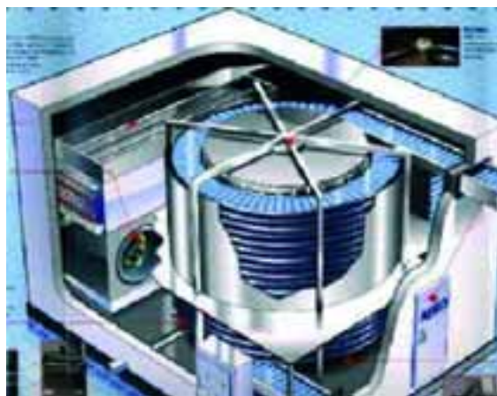
Figure 8. The cross-section view of a spiral belt freezer.
