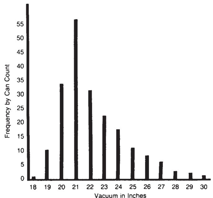
FIG. 2.†. HISTOGRAM FOR VACUUMS IN CANNED SOUP
