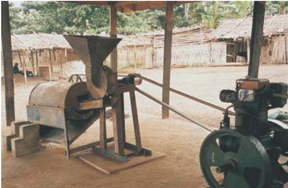
Fig. 19 Palm nut cracker combined with Kernel/Shell separator (Hormeku Engineering works, Ghana)
