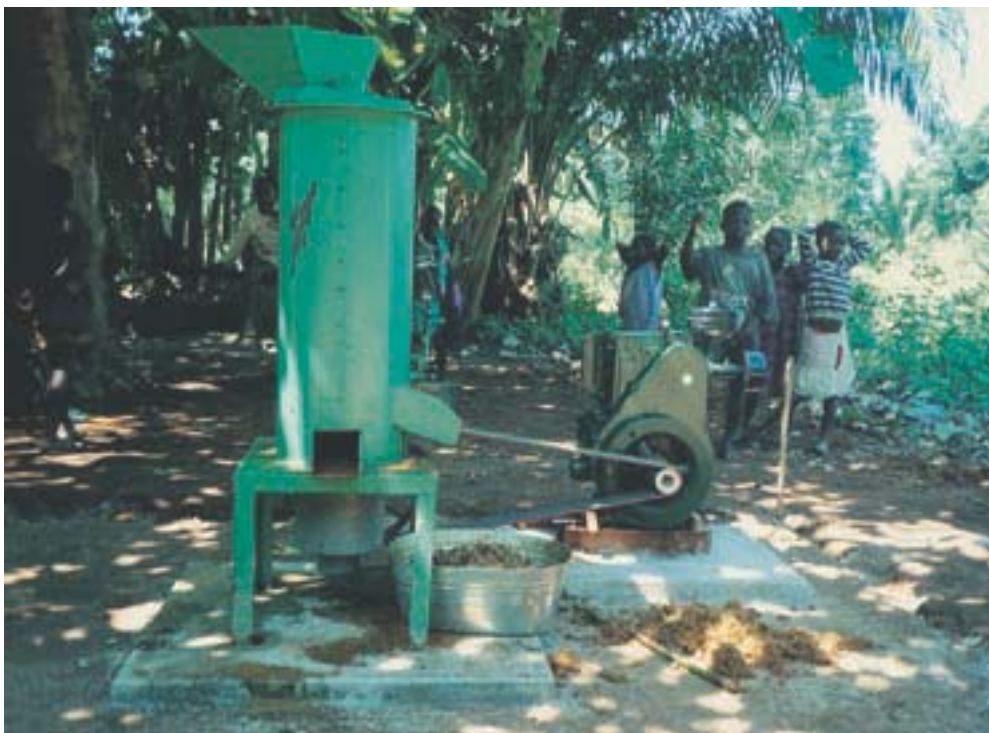
Fig. 12 Flushing extractor (Cort Engineering Services, Ghana)
