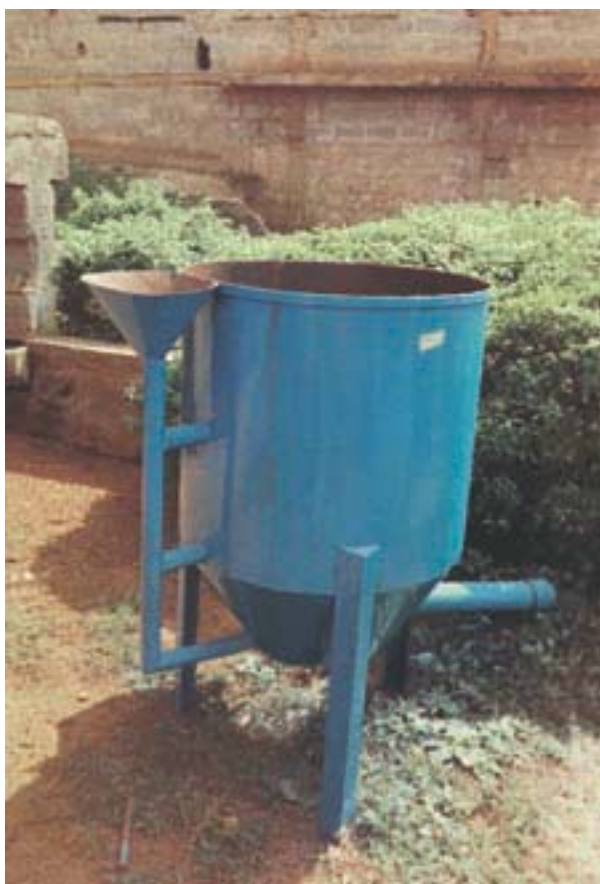
Fig. 14 Clarifier tank (Nova Technologies Ltd, Nigeria)
