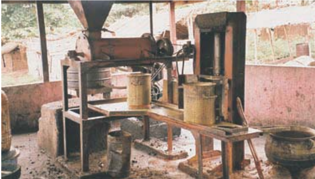
Fig. 11 Combined digester and motorised hydraulic press (Technoserve/Cort Engineering, Ghana)
