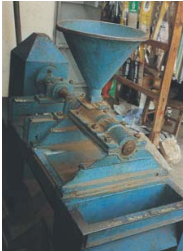
Fig. 20 Whole palm kernel expeller (CAMEMEC, Benin)
