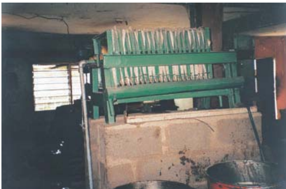
Fig. 15 Oil filter (Faith Engineering Workshop, Nigeria)
