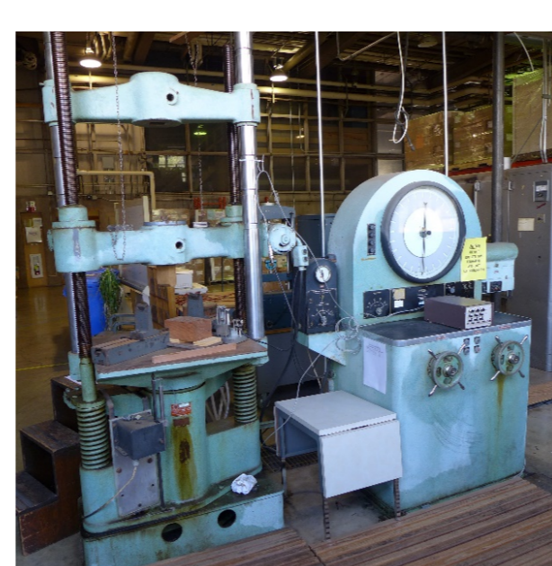
Figure 1: Baldwin 60,000 Universal Testing Machine
