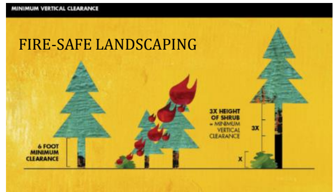
Photo above (courtesy of CAL FIRE) shows a 5' shrub near a tree. In this example, 15' of clearance (3 x 5') is needed between the top of the shrub and the lowest tree branch to prevent a fire ladder.
