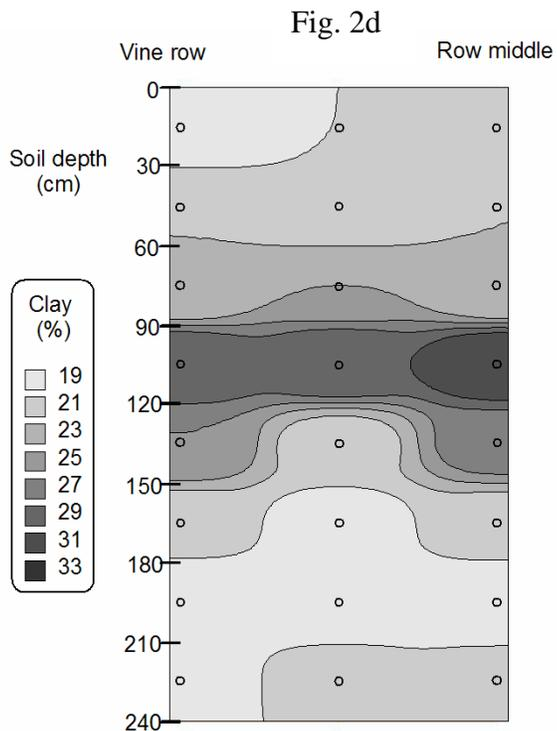
Figures 2a-d. The soil  $EC_e$ , exchangeable sodium, extractable boron, and percentage clay, as vine row soil cross-sections at the 2010 site with the highest salinity levels. Drip irrigation is applied only in the vine row. Each 30 cm depth increment is equivalent to 1 ft. The distance between the vine row and row middle was 4 feet at this location.
