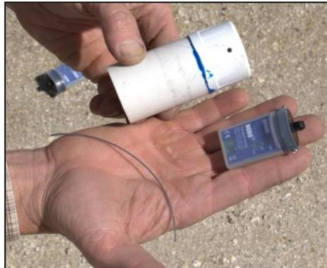
In this example, the shield for the lower datalogger has an additional "saddle" piece made from 1-1/2" PVC pipe glued to the side; this may help it attach more securely to the steel line post. This is optional.
