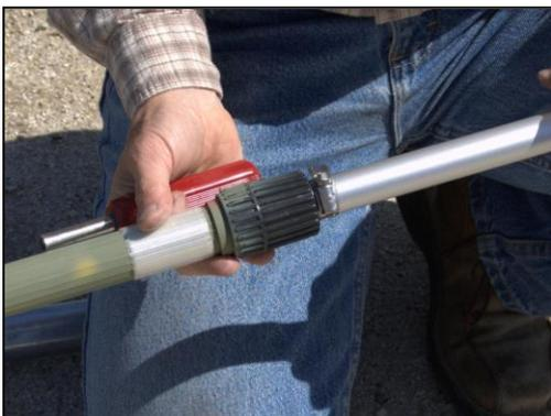
Fully extend the lower extendible aluminum pole section from the “Mr. Longarm.” Once fully extended, retract it one foot back inside the fiberglass section. This is important to do, as it provides additional support at this potential weak point. Tighten the black plastic lock by hand.
