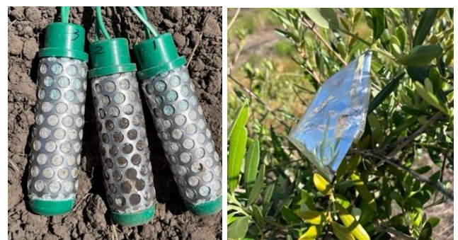
Tools to assess soil and plant water status: soil moisture probes (left), stem water potential (right).
