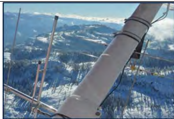
Illustration D6: Forest Service Cessna 185 airplane, and antenna configuration on the right side wing strut.
