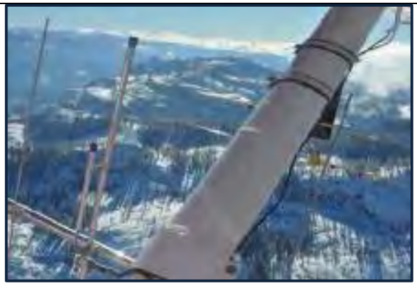
Illustration 7: Forest Service Cessna 185 airplane, and antenna configuration on the right side wing strut.
