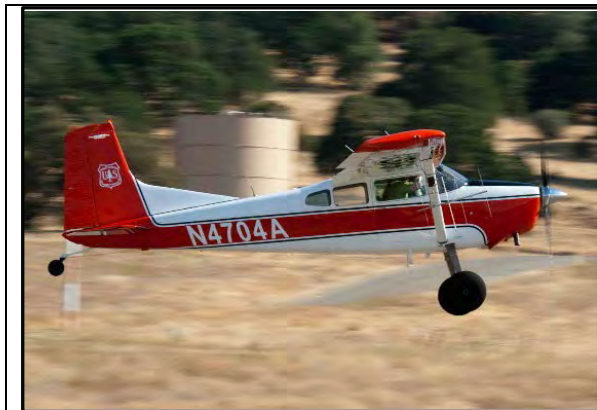
Illustration D6: Forest Service Cessna 185 airplane, and antenna configuration on the right side wing strut.
