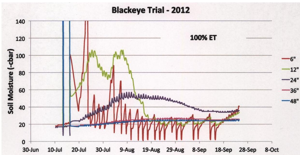
Figure 2. 2012 season soil moisture levels in the 100% ET irrigation treatment. The soil moisture was monitored using Watermark soil blocks connected to a Watermark data logger.
