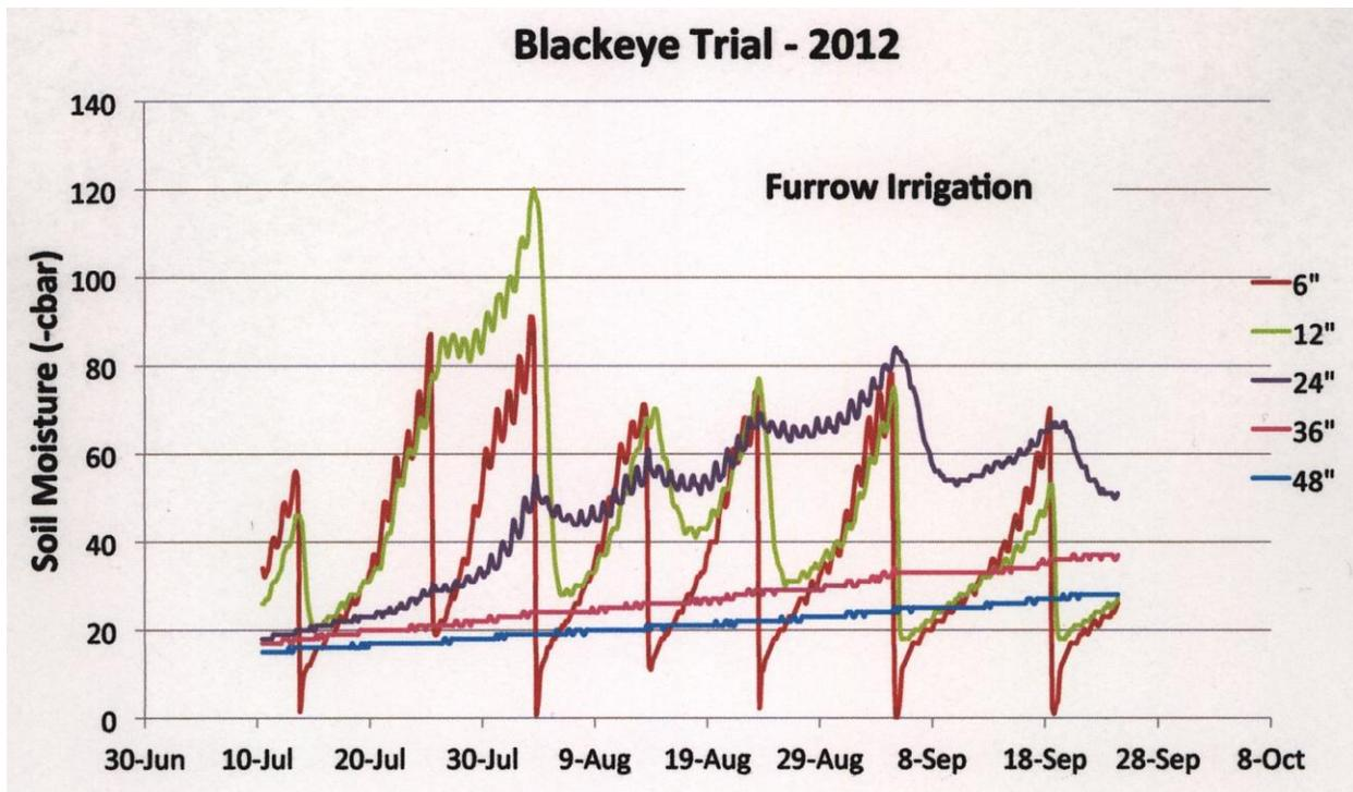
Figure 5. 2012 season soil moisture levels in the furrow irrigation treatment. The soil moisture was monitored using Watermark soil blocks connected to a Watermark data logger.
