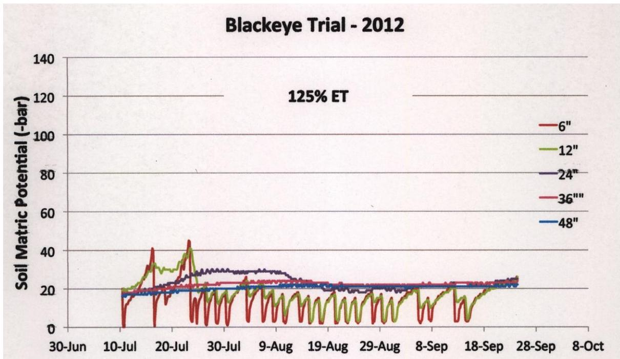
Figure 4. 2012 season soil moisture levels in the 125% ET irrigation treatment. The soil moisture was monitored using Watermark soil blocks connected to a Watermark data logger.
