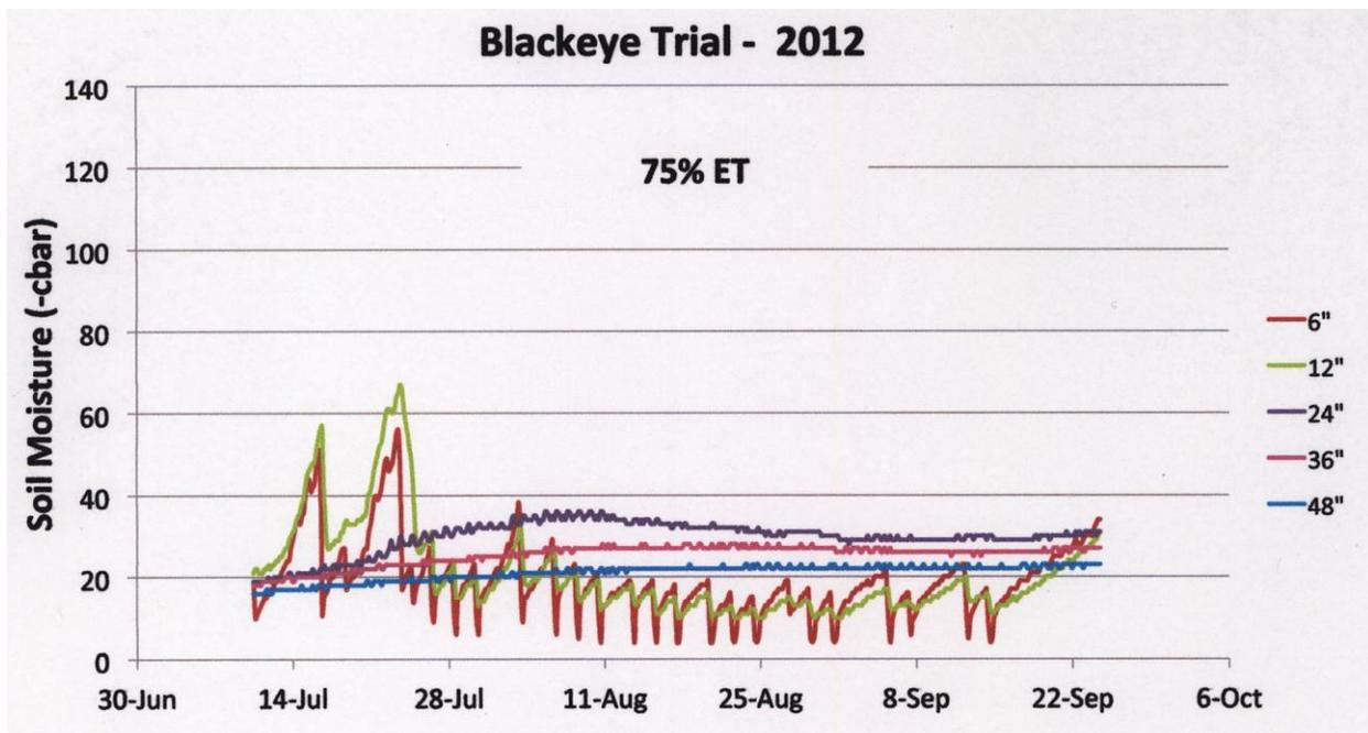
Figure 1. 2012 season soil moisture levels in the 75% ET irrigation treatment. The soil moisture was monitored using Watermark soil blocks connected to a Watermark data logger.
