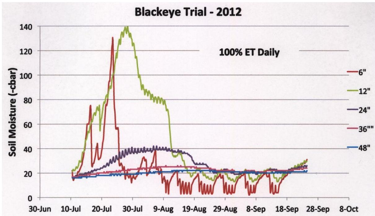
Figure 3. 2012 season soil moisture levels in the 100% ET, daily application irrigation treatment. The soil moisture was monitored using Watermark soil blocks connected to a Watermark data logger.
