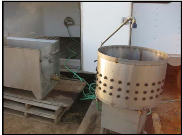
The processor's scalding and plucker is all set up to process turkeys at Natural Trading Company in October 2009.
