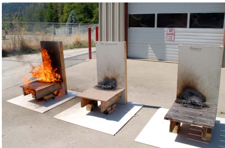
Figure 3. A photograph of a fire demonstration showing differences in performance between three different decks. From right to left, a solid untreated redwood deck (complies with code requirements), a wood plastic composite product (complies with code requirements), and a wood plastic composite product (non-compliant). All decks were initially subjected to a burning ASTM Class B placed on top of the deck. This photograph was taken approximately 30 minutes after the start of the test.
