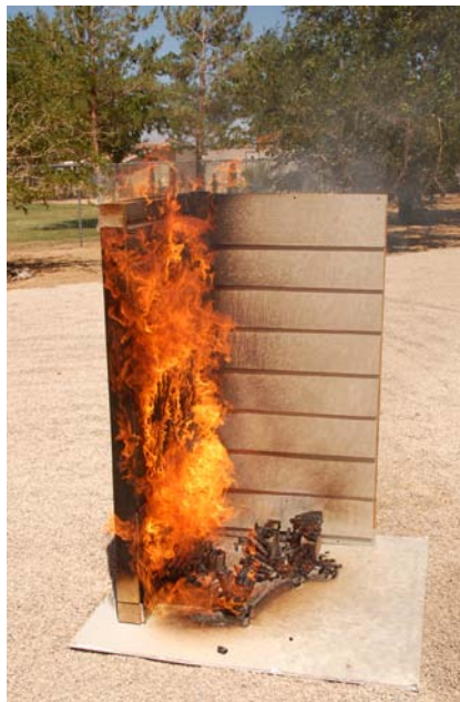
Figure4. A photograph of a fire demonstration using a wall corner section. A hardboard siding product (left, burning) and fiber cement product (right, not burning) were subjected to a burning American Society of Testing and Materials (ASTM) E-108 Class A brand, placed at the base of the wall. The test standard for siding does not directly evaluate flame spread.
