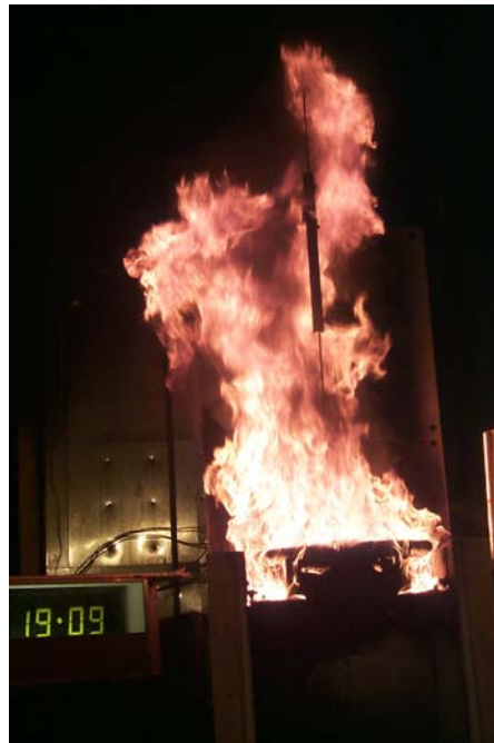
Figure 2. A plastic deck product subjected to the under-deck flame contact exposure test described in SFM 12-7A-4. The flame exposure lasts three minutes. As formulated, this decking product would not meet the heat release rate requirement and therefore would not be approved for use in wildfire prone areas.
