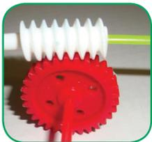
**Worm Gear** – good for gear reductions as they have one spiral groove or tooth. They also have a locking quality in that the worm can easily turn the driven spur gear but the spur gear cannot make the worm turn. This is a good way to hold robot arms, wheels, or other gears in place or position.
