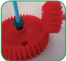
**Bevel Gear** – useful to change direction of the rotating shafts — usually at 90 degrees — but some are made for other angles.
