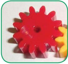
**Pinion gear** – usually a small gear used as a driver. It may be attached directly to a motor.
