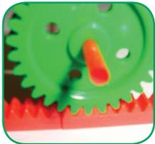
**Rack Gear** – can be used to convert rotation motion into linear motion, or vice versa, either with the rack moving or the pinion moving across the rack.
