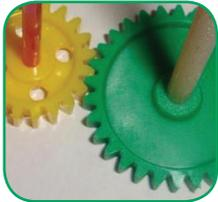
**Spur Gear** – the most common type of gear. Different size diameter gears are used together in a set to change speed or rotation direction.
