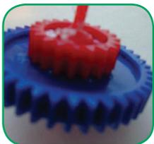
**Compound Gear** – two or more gears of different sizes (diameter) connected so they rotate together either on one shaft or as one piece. Used to compound or increase the gear ratios in changing rotational speed or ratio.
