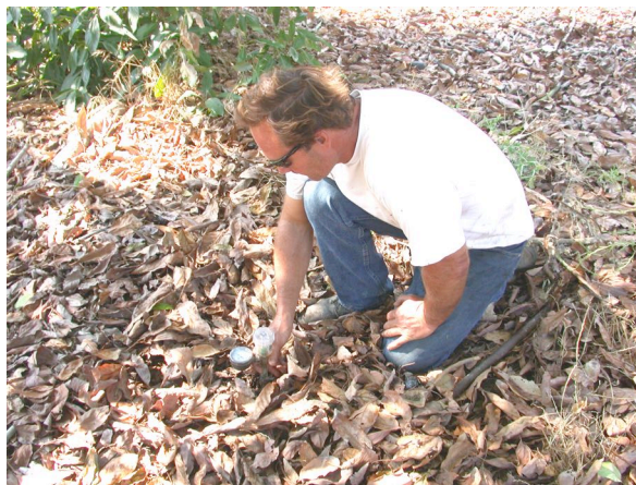
Figure 1. Reading a tensiometer, a key to irrigation scheduling.
