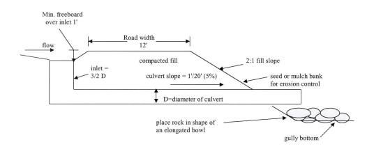
Figure 3: Profile of Culvert Installation
