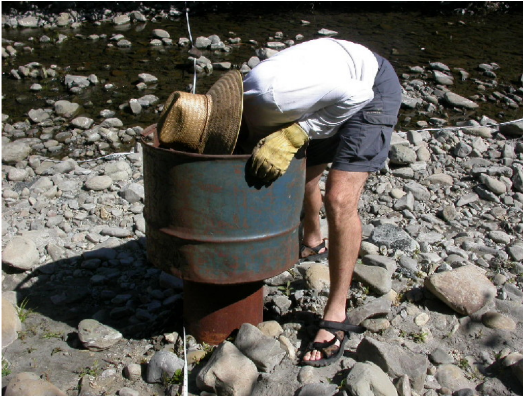
Figure 19. Bulk Sampling With Barrel Sampler.
