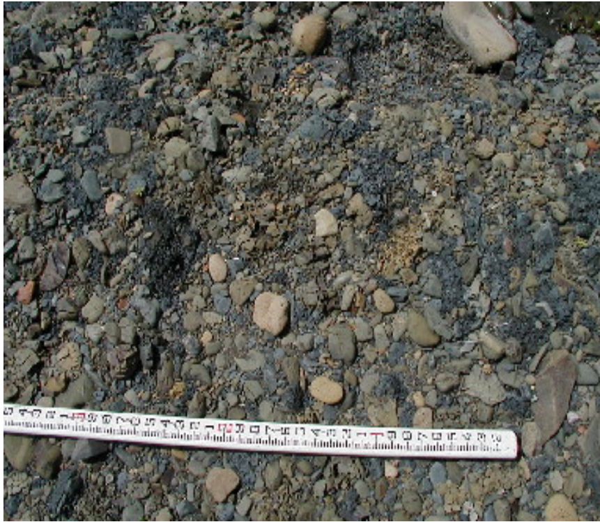
Figure 14. Sampling Surface Substrate Size Using the Pebble Count Method. Pebbles are selected for measurement at systematically determined intervals.
