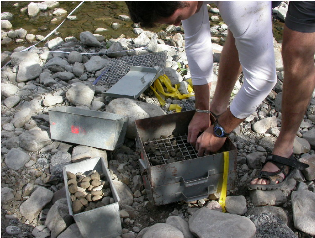
Figure 20. Field Processing of Bulk Samples.
