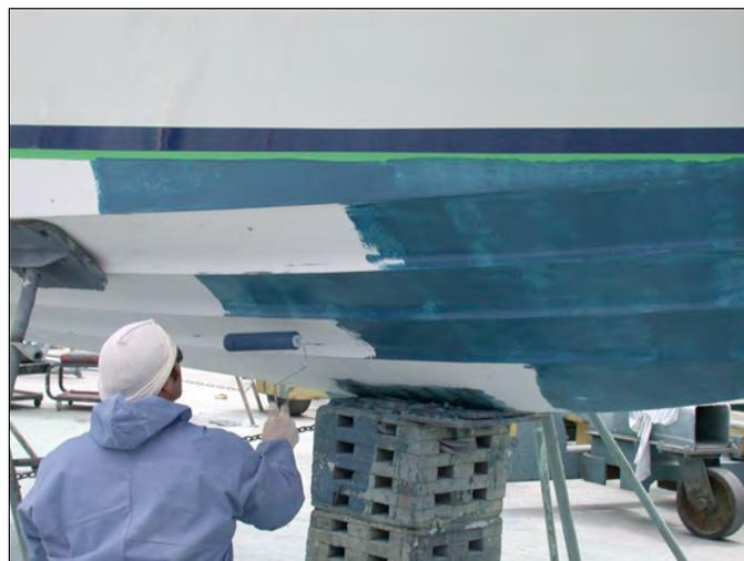
Applying nontoxic coating to boat hull
