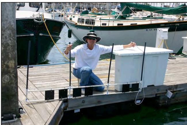
“Continuously cleaned” panels were cleaned in water for three months using California BMPs. “Cleaned once” panels were cleaned only at the end of three months. Then, both sets of panels were redeployed for a fourth month, and a set of new “not cleaned” panels was added.
