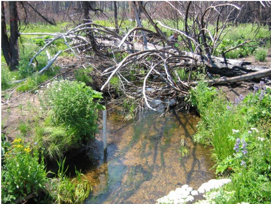
Figure 4. Angora Creek channel monitoring station with staff plate and bank scour pins.
