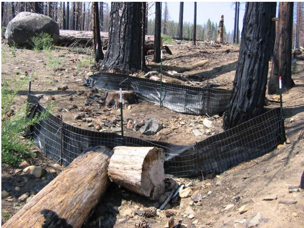
Figure 8. Silt fences installed in an ephemeral tributary channel of Angora Creek to measure sediment contribution from the treated hillslopes.
