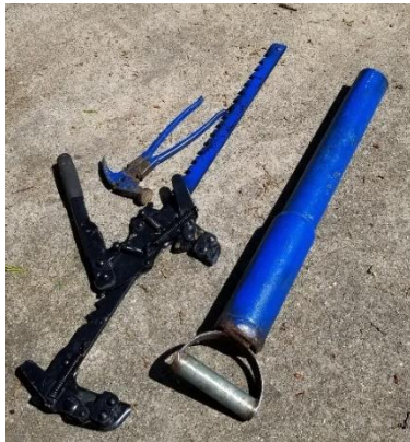
Figure 2: Modified T-Post Driver for the Mountains
