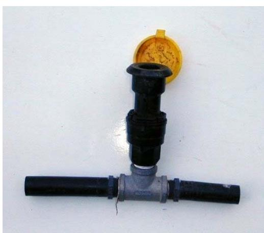
The design for this portable system comes from Kentucky Graziers Supply (800-729-0592). This system uses a quick coupler hydrant in the main line and has a trough that holds 60 gallons. There are other troughs of smaller size. If you have adequate recharge (4 gallons per minute), you can get by with a larger trough. Ralph Quillan owns the company and he uses these products on his own farm. He has been able to water 100 head with a 14 gallon trough!.
