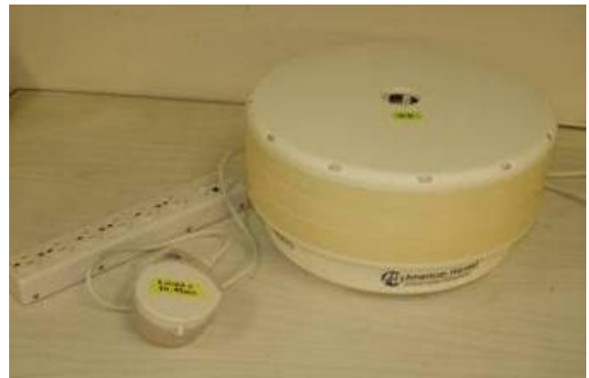
Picture 1. Dehydrator: Nesco/American Harvest Snackmaster® Pro Food Dehydrator Product No. FD-50 http://nesco.com ($59.95). Automatic timer: GE 7-day home Security Timer DESC.: GE5112N-71M4SP Kmart ($7.99). 6 Outlet Metal Surge Protector: Power Sentry or comparable, Walmart ($12.77).
