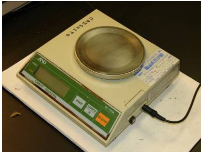
Picture 2. Balance, comparable to Denver Instrument Model MXX-212 with a capacity of 210 g, readability of 0.01 g, taring range of 0-210 g.
