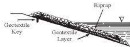
a. Filter Behind Riprap for Stream Bank Protection.
