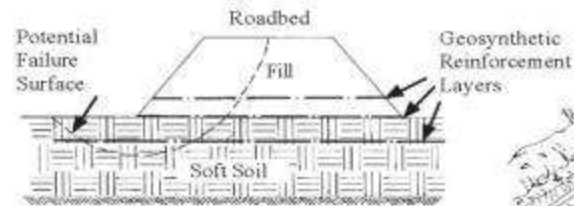
c. Embankment Reinforcement over Soft Soil Deposits
