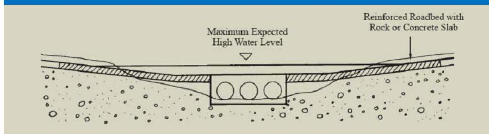
b. Improved (Vented) Ford with Culvert Pipes in a Broad Channel
