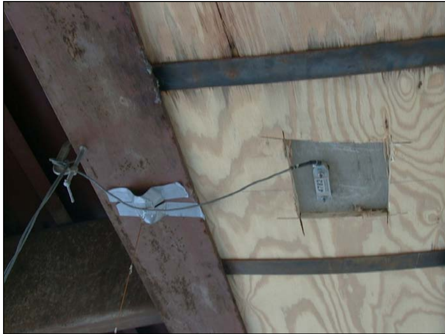
a. Strain transducer on concrete longitudinal RRFC connection.
