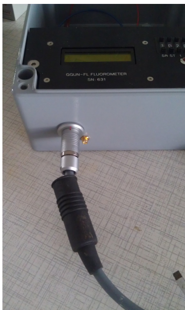
Figure 1: Cable connection to the FL30 logger box.
