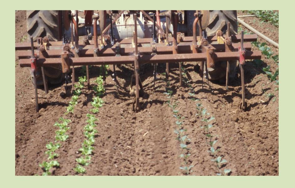
Two row cultivator utilizing sweeps and knives and chisels
