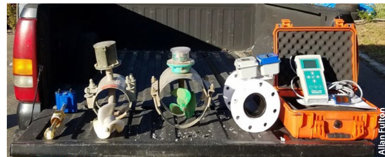
Figure 8. Examples of flow meters that can be used in irrigated agriculture. From left to right, an insertion paddle wheel meter, two impeller meters, a magnetic meter, and a Doppler meter.
