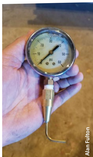
Figure 3. The photo shows a 60 psi liquid-filled pressure gauge connected to a brass pitot tube. This can be used to measure pressures in lateral lines and at nozzles of microsprinklers and solid-set sprinklers. Pressure measurements can be compared with technical information for specific emission devices (an example is on the right) to determine how much the pressure variation may be affecting water discharge rates and irrigation uniformity. A 15 psi or 30 psi pressure gauge would be more appropriate for drip irrigation systems. Source: Allan Fulton.
