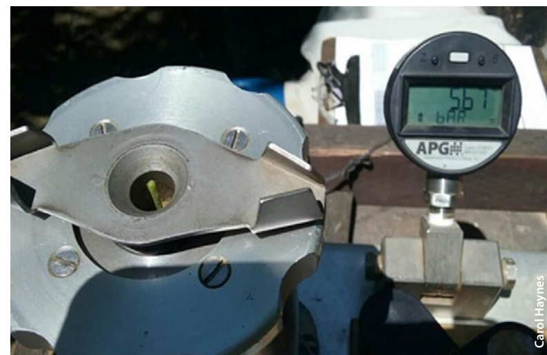
Figure 14. Photo of actual SWP measurement in walnut using a pressure chamber with a digital gauge. Plant water status of this walnut tree was -5.67 bars tension. Photo: Carol Haynes.
