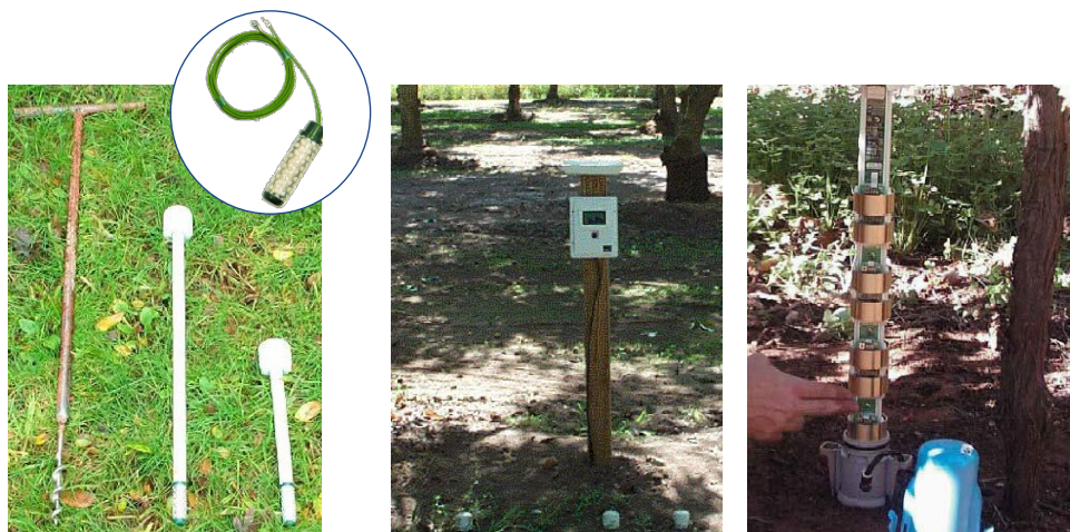
Figure 10. Two types of soil moisture sensors. Left and middle: Watermark resistance sensors with a datalogger; right: one type of dielectric soil moisture sensor. Source: Watermark photos: Allan Fulton; Dielectric sensor photo: anonymous.
