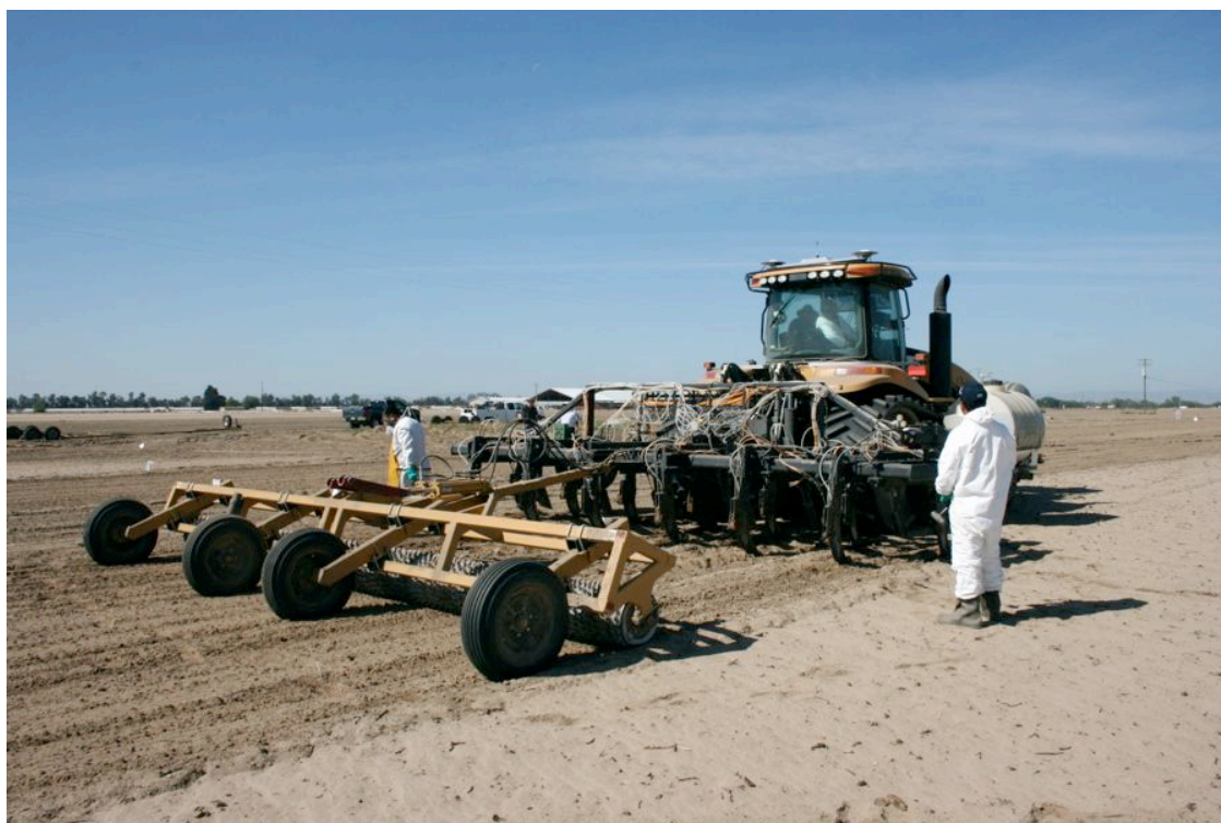
Figure 1. Spring fumigation injections. All treatments were shank applied, and then the soil was sealed with the ring roller.
