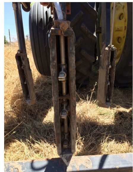
Figure 1. Emitters within each shank were at 3, 6, and 9 inches.
