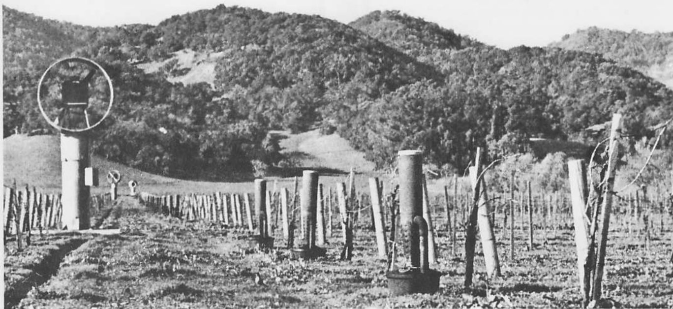
Fig. 2. This movable wind machine is situated in a vineyard avenue. Note two similar machines in the background, and the placement of return-stack heaters.
