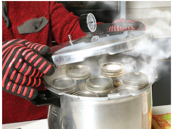
Figure 21. After cooling the canner, open the vent port. Wait 10 minutes; then open the canner, lifting the lid away from you so the steam does not burn your face or arms.
