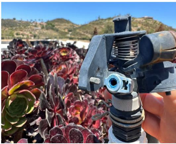
Figure 2. Specifications for the Rain Bird 2045PJ "Maxibird" impact sprinkler. Note the blue nozzle in figure.
