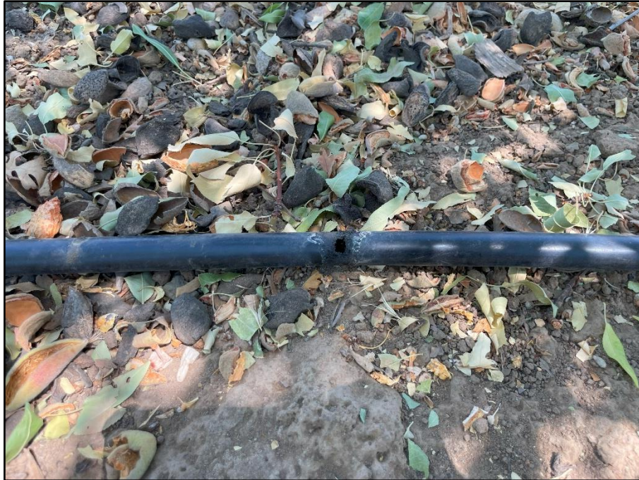
Irrigation dripline damaged by ground squirrels. (Photo: C. Reyes)
