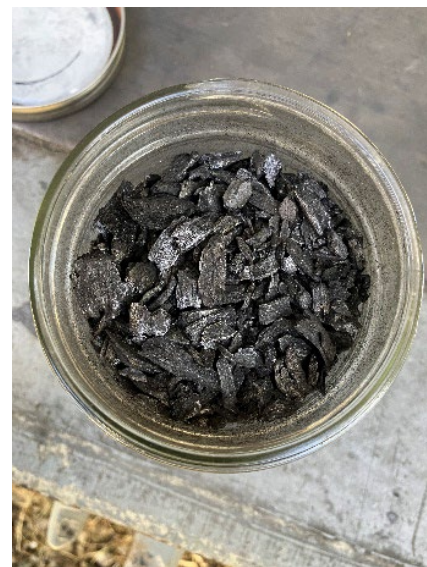
Figure 2 Jar of biochar made as a byproduct from bioenergy production.
