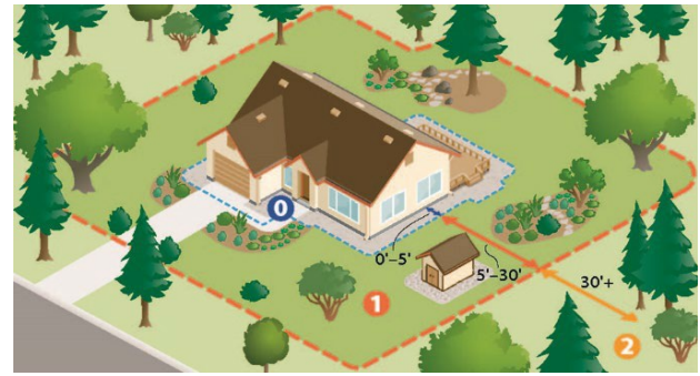
Figure 5: California's 3-zone defensible space system is critical for fire mitigation.
