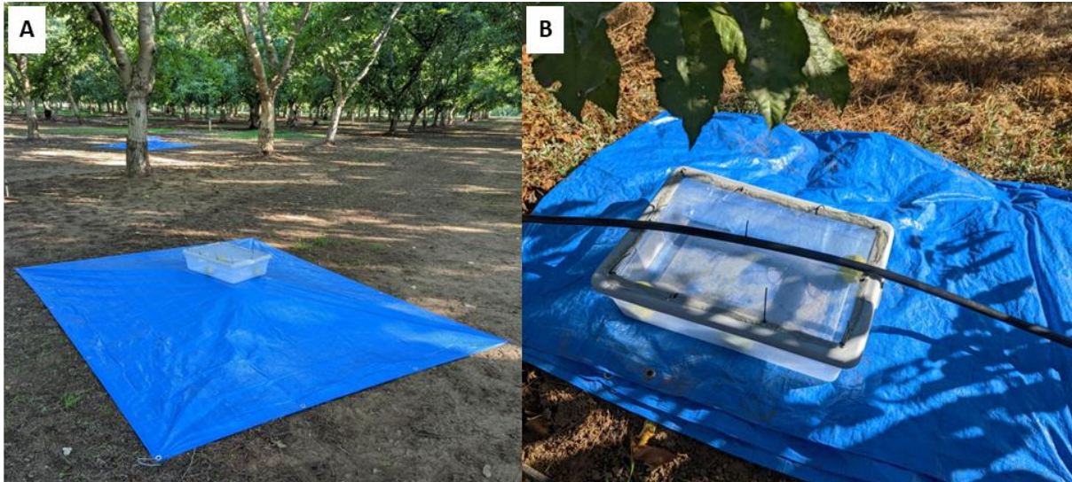
Orchard sampling stations used to detect live Phytophthora in water from A , sprinklers and B , drip emitters.
