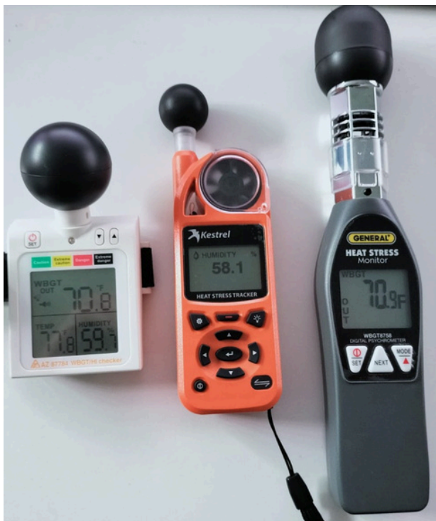
Portable heat-stress measuring instruments for testing & education. Photo: K Bharambe
