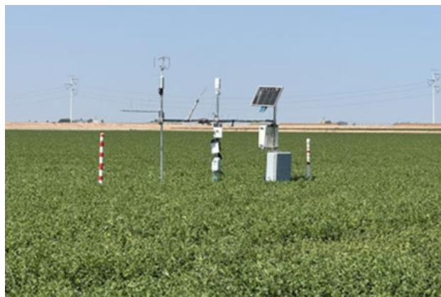
Figure 2. Eddy covariance tower and soil moisture monitoring installed in a representative alfalfa field in the Imperial Valley, used to measure crop water use and soil water conditions in the field.
