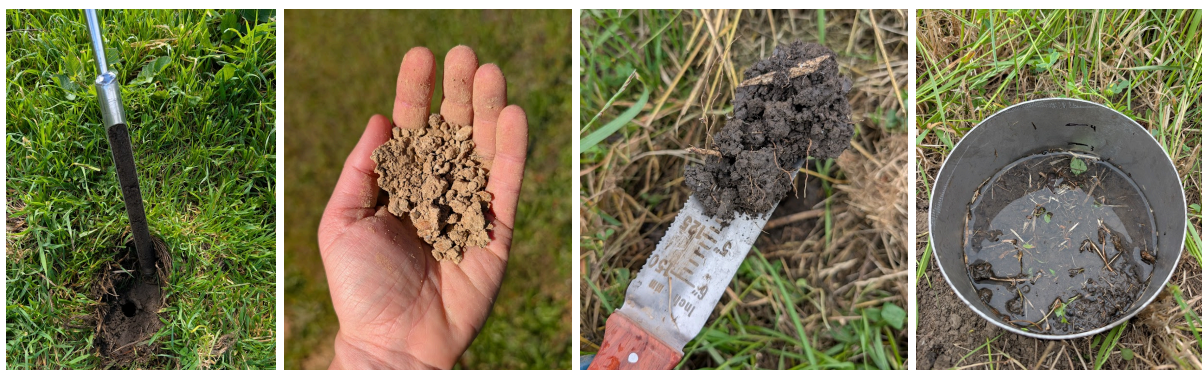
Fig 2. From left to right: soil sampling using soil probe, upland vineyard soil, lowland cover crop soil, soil water infiltration testing.
