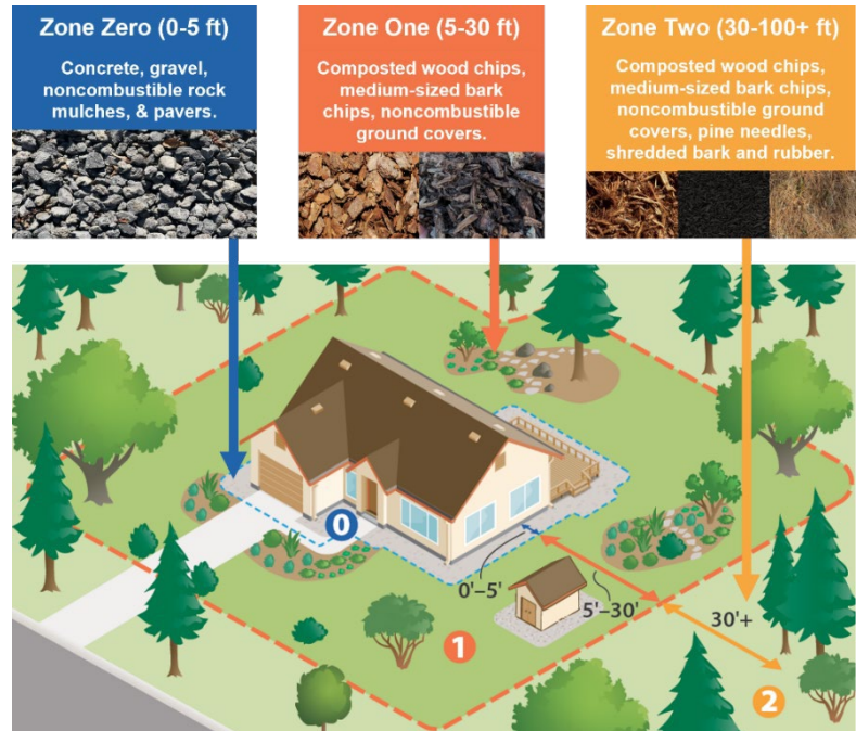
Figure 1: Examples of how different types of mulch can be integrated into a near-home defensible space strategy. 11
