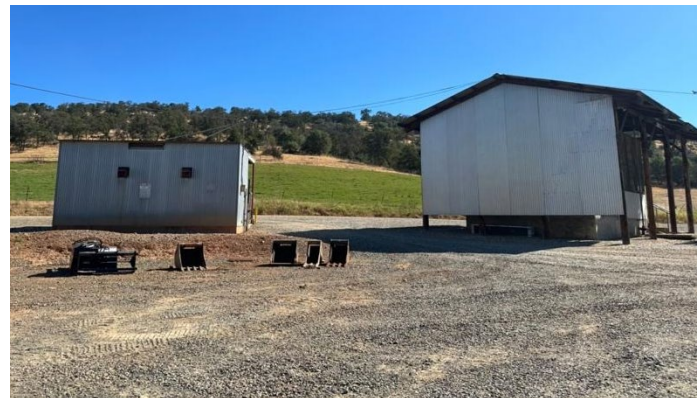
Figure 9: Defensible space zones may overlap. Consider looking at building footprints as one larger structure and implement your Zone One or Two strategies accordingly.
