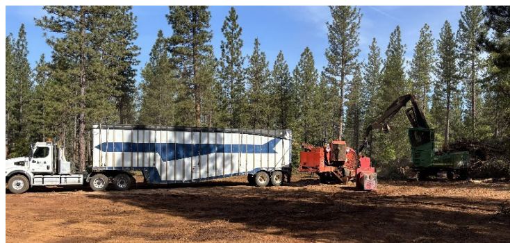
Figure 3: A chip van being loaded at a landing. PC: Evan Watson
