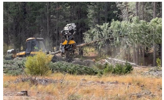
Figure 1: A feller-buncher holding a recently harvested tree. PC: Hunter Noble
