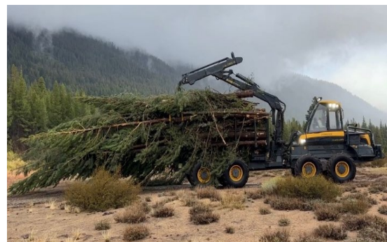
Figure 2: A forwarder transporting recently harvested trees to the landing. PC: Hunter Noble
