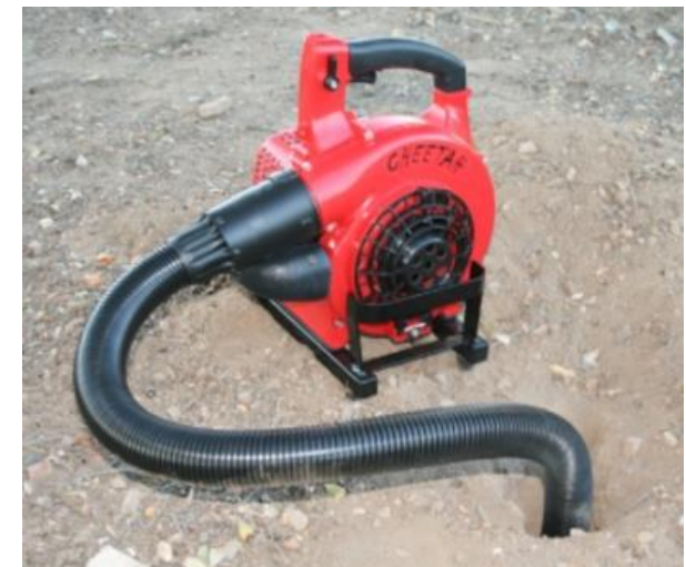
Pressurized Exhaust System
