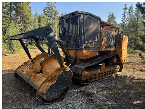
Figure 2: Tracked masticator with front-end mounted drum cutting head. Photo: Amber Lennon
