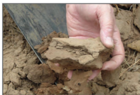
Photo 1. Compacted soil from a main skid trail indicating that the skid trail may have been used during suboptimal soil conditions.
