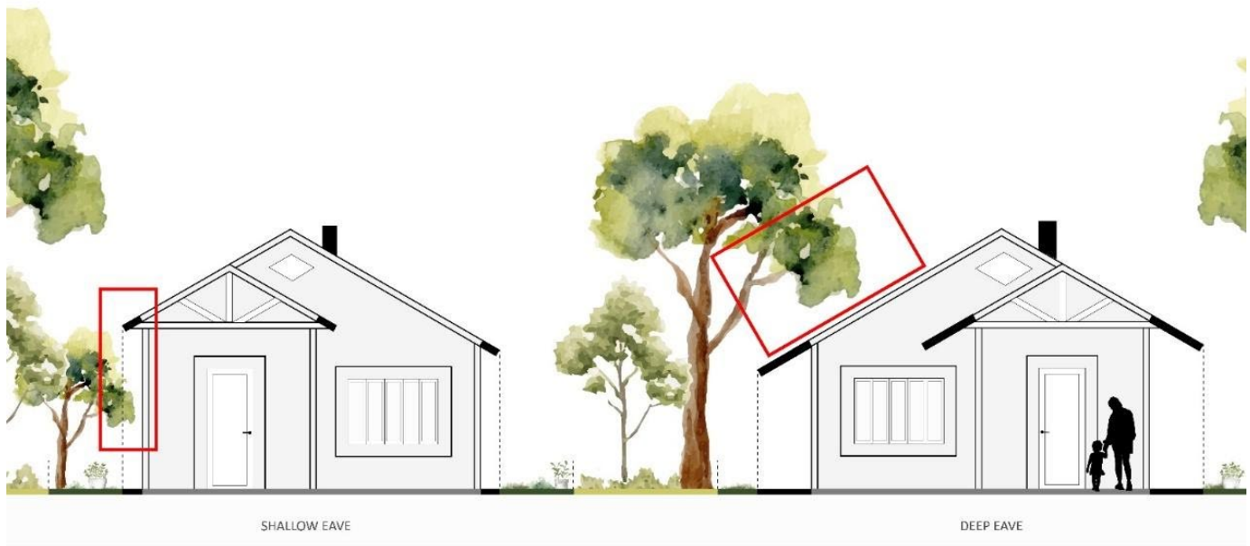
Figure 2: This illustration shows trees within Zone 0. On the left is a young tree with most of the ladder fuel removed, but a few smaller branches remain under the eaves and would need to be trimmed as indicated by the red box. On the right side, a larger tree is very close to the roof. While the lower ladder fuels are removed, an inspector would suggest removing one limb to provide 5 feet of clearance between tree limbs and the roof, reducing the risk of fire transmission to the roof. The recommended trimming area is indicated by the red box on both trees.
